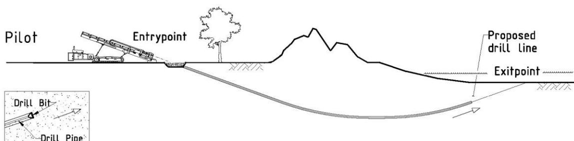
4.13 A wider working area of 50m is needed where HDD is to be utilised than where trenched installation methods are used. This is because:
