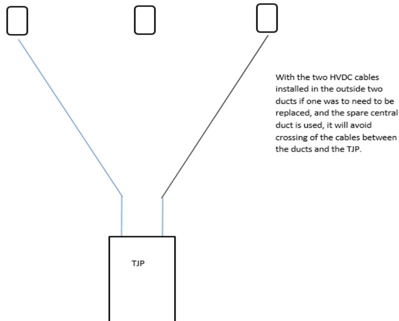
4.11 The submarine cables will terminate at a buried TJP located inland of the existing sea defences to the west of Roman Bank, where they will connect to the underground onshore cables.
