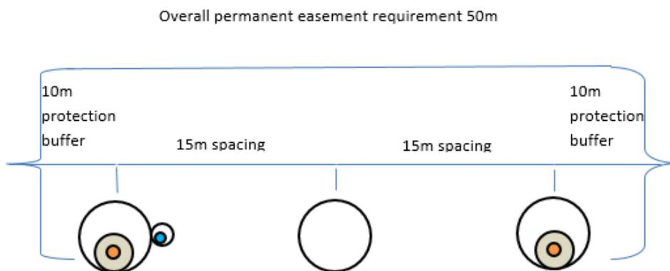
Cross sectional view towards the sea of the four (4) ducts. The submarine power cables will be installed in the outer two ducts with the submarine fibre optic installed adjacent to one core
