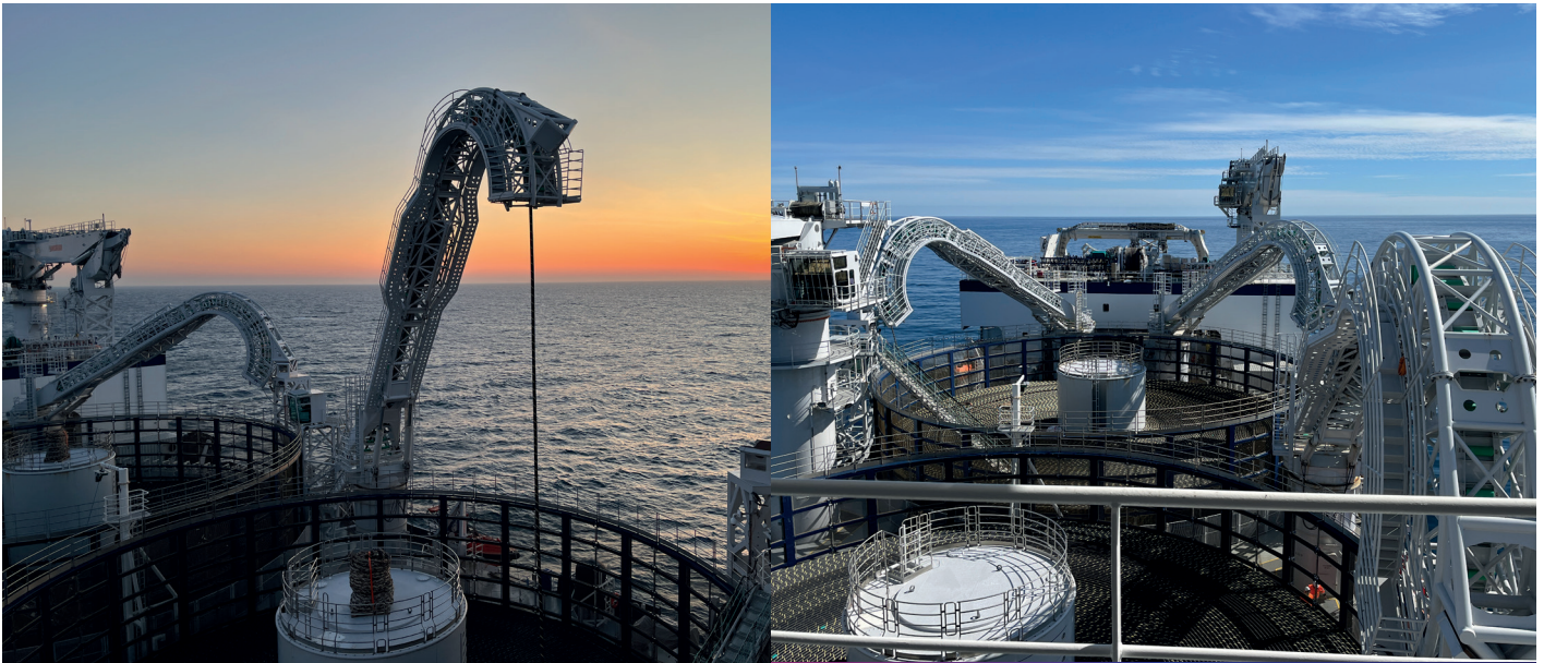
Images from the Leonardo da Vinci laying Viking Link's offshore cable
