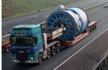
Cables are transported to site on special low loader vehicles
